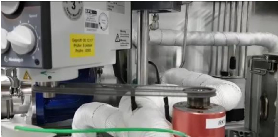
Figure 6. Stirrer using a belt that worked through toothed wheels.
