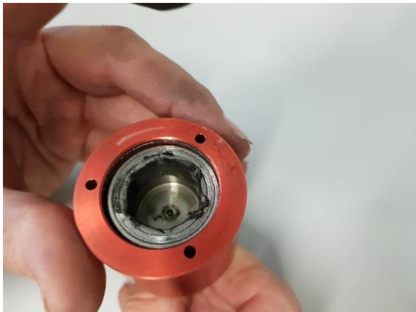
Figure 7. Ball bearing repair.
